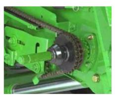
Feed Accelerator Speed Slow side speed - 430 rpm Inner Large Diameter
